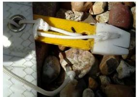
Tensioning is by the notch, which rarely comes loose, but also tie 2 figure of eight knots in the line, as per photo. The first is to prevent the batten end from coming off, and the second is to assist your grip when tensioning.
